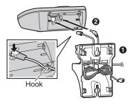
3 Insert the hooks on the wall mounting adaptor into the holes **(A)** and **(3)** on the base unit.
